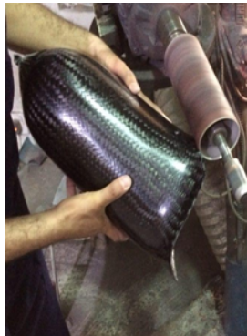
Figure 5. Cutting and smoothing for manufacturing (AK).
