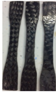
Figure 2. The general shape of tensile specimens.
