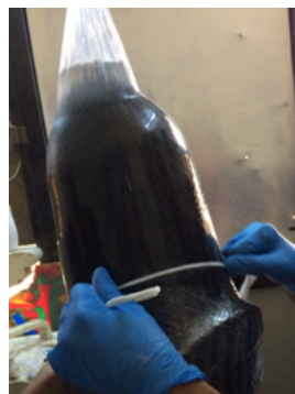
Figure 4. Lamination used for manufacturing (AK).
