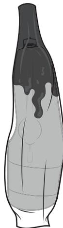
11 If doing two stage lamination, transfer socket alignment now.
