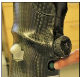
White tether release button and green tether draw button on a release/relock socket.
